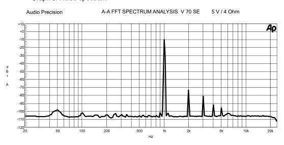
Noise spectrum at 1 kHz / 5 W into 4 ohms – there is no mains interference to be seen. (50 Hz < 200  $\mu$ V, 100 Hz < 70  $\mu$ V) The k2, k3, k4 and k5 noise spectrum is extremely low and falls quickly.
