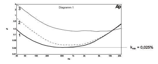
Curve 1: BIAS adjusted correctly
