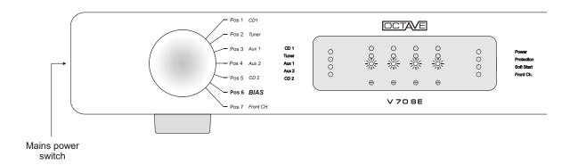
Five LEDs will now illuminate: The power LED and the 4 BIAS LEDs in the center of the display, one for each power tube. If the amplifier is still cold, the LEDs will initially illuminate "yellow".
